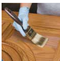
Step 3: Seal with top coat.
